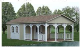
**Standard Features: Vinyl sided:** 6'dbl. steel door 11 lite glass, 3'steel door 11 lite glass, 30 year architectural shingle, 6 pitch roof, gable overhangs, two 24x36" windows w/ shutters, miratec trim board on rake & face. **Vinyl Porch:** composite evergrain decking, (gray, weatherwood, redwood & cedar), top & bottom vinyl rails, balusters and vinyl ceiling. Screen porch includes a door and screening under deck.
